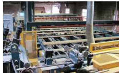
Use of a Lico optimizing rip system measures each board, determines the best cutting pattern for each, and utilizing a moving arbor rip saw, can cut any combination of flooring blanks in the various widths the company produces.
